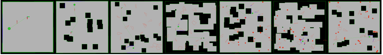
Fig. 3: Stage one to seven of the 2D simulator on our arena-rosnav platform [5]. The maps increase in difficulty by adding more static and/or dynamic obstacles to it.
