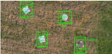
Fig. 11. Example of figures detection with YOLOv5 algorithm, during Droniada 2021
