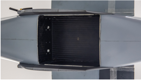
Fig. 7. HF-10 SZCZYGIEL VTOL payload bay
