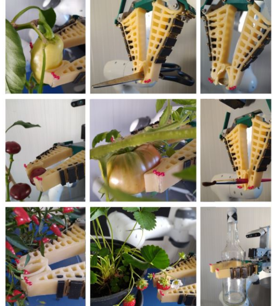
Fig. 1: SofIA soft gripper mounted on FRANKA EMIKA Panda robotic arm handling fruit and vegetables (peppers, tomato, and strawberry) and miscellaneous everyday objects (a bottle, a coin, a paintbrush, scissors) in both horizontal and vertical approach. The serial chain hinge support is mounted on the outer side of the Fin-Ray finger structure.
