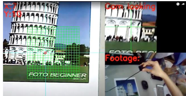
Fig. 1. The positioning DCN compares a base image with the real-time cam image to predict precise coordinates of the cam position.
