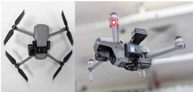
Fig. 2. DJI Air 2 with INSTA360 Sphere Camera. Top View (Left) and Side View while flying (Right).
