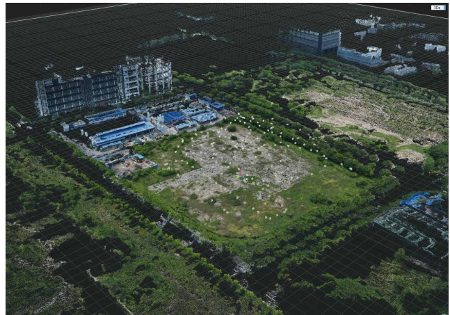
Fig. 3. Image Alignment and 3D Reconstruction.
