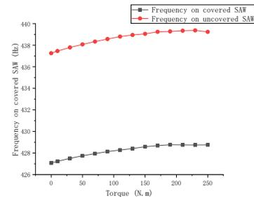
Fig 4 Comparison of frequency changes between covered SAW and SAW
