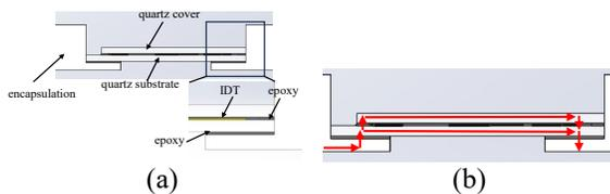
Fig 2 (a) SAW wafer package structure;(b) SAW encapsulated force transmission direction
