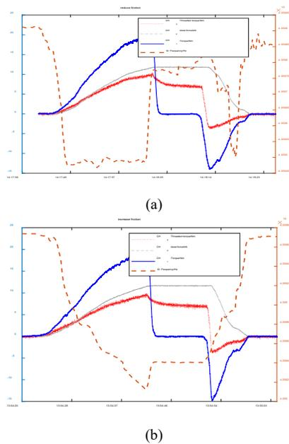
Fig 11 (a) reduced friction on the bottom surface of the gasket (b) increase friction on the bottom surface of the gasket
