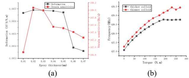
Fig 6 (a) Effect of colloid thickness variation on wafer deformation and strain sensitivity;(b) Comparison of SAW frequency changes for thinner and thicker colloids
