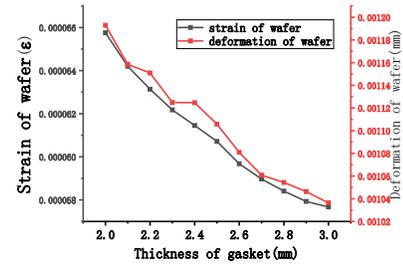
Fig 8 Simulation of the effect of shim thickness on wafer deformation and strain
