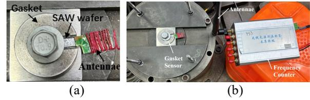
Fig 7 (a) Sensor's structure & Antennas; (b) Experimental equipment and connectivity
