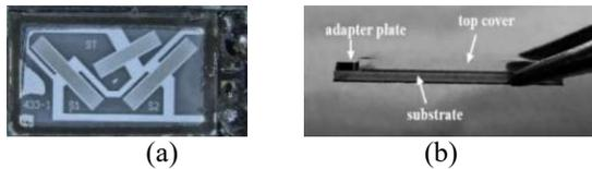
Fig 1 (a) 433MHz SAW unit;(b) Saw unit composition
