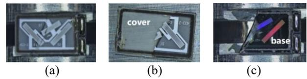
Fig 3 (a) SAW lower fragmentation figure; (b) SAW upper cover adhesive part lower substrate;(c) SAW section lower substrate
