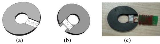
Fig 9 (a) Schematic of 6mm slotted spacer sensor;(b) Schematic of 10mm slotted spacer sensor;(c) 10mm slotted gasket with antenna
