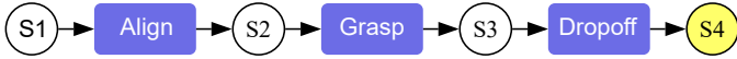
Fig. 4. Petri Net representing the example plan reported in § III. The state reported is the final step, when one Token is state s_4
