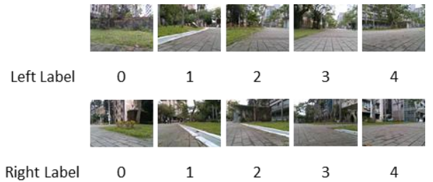
Fig. 4. These images are samples used to train the left and right TRAC models, which were captured by the single camera mounted on the robot.
