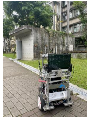
Fig. 1. To conduct map-free autonomous navigation in unstructured outdoor environments, the proposed system employs GNSS and compass to track the destination's location, while the Traversable Region Abbreviation ConvNet provides the real-time field information for movement controls.
