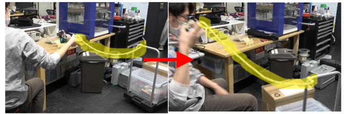
Fig. 8. Total demonstration of the prototype after integrating all system. Holding ability was enhanced by tightening after twining around the dolly handle and enable user to pull the dolly.
