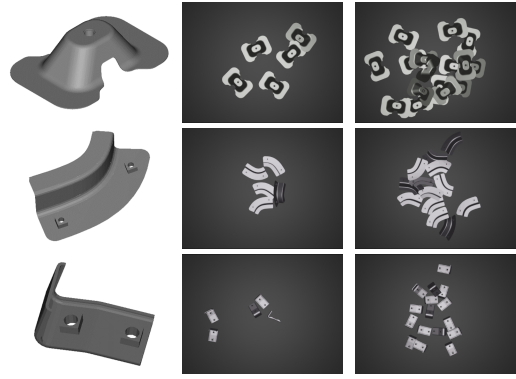
Fig. 6. Three kinds of sheet stamping parts and some simulation scenarios.
