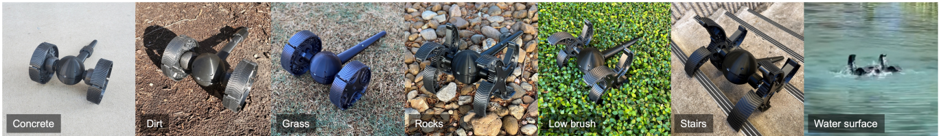
Fig. 5. Locomotion testing environments including concrete, dirt, grass, rocks, low brush, stairs, and water.
