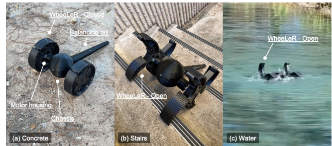
Fig. 1. ARMoR with passively transforming wheels on (a) concrete, (b) stairs, and (c) water surface.
