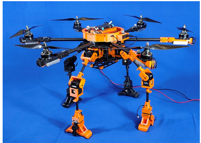
Fig. 1. Multi-limb morphogenetic UAV for aerial manipulation and terrestrial locomotion
