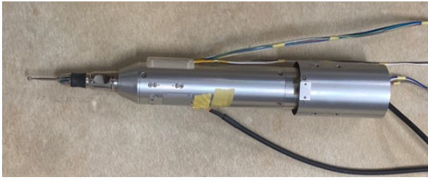
Fig. 1. Proposed orthopedic haptic drill
