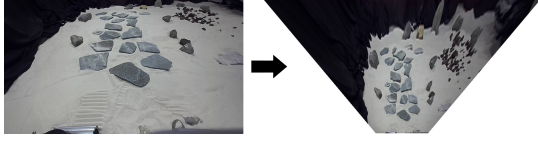
Fig. 2. Homography transformation to convert the coordinate.
