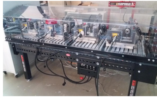
Fig. 1. Fleet of 4 bearing health monitoring setups at the Flanders Make lab [17]. A second identical test rig is present with 3 more setups.
