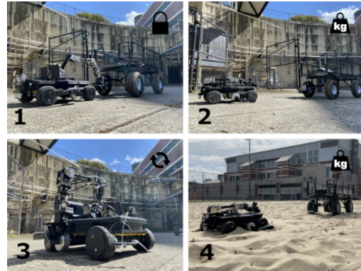
Fig. 1. (1) Vehicle-mounted manipulator can localize and attach the payload to the vehicle. (2) An anchoring device can be engaged on a given surface to increase payload capacity. (3) The anchoring device can be swapped using the manipulator for a different surface. (4) The robot can pull the payload on a different surface using a different anchor.
