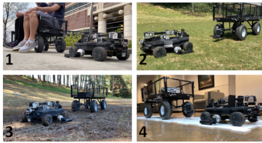
Fig. 10. Terrain testing across multiple surfaces. (1) Microspine anchors pulling up to 265kg on concrete. (2) Microspine anchors pulling up to 115kg on grass. (3) Macrospine Anchors pulling up to 115kg on mud. (4) Adhesive-rubber anchor pulling up to 195kg on polysynthetic ice. Sand Anchors pulling up to 60kg is shown in Figure 1.
