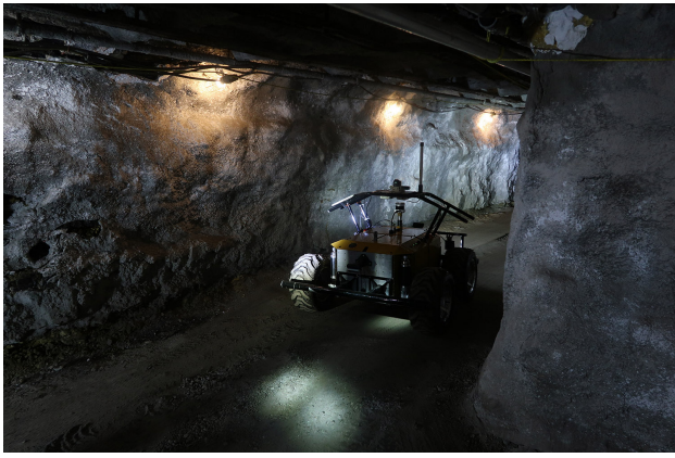
Fig. 6. Rhino Robot inside the experimental Mine while mapping.
