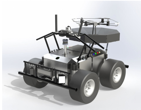
Fig. 2. Rhino robot rendering, including sensors, landing platform, and the drone
