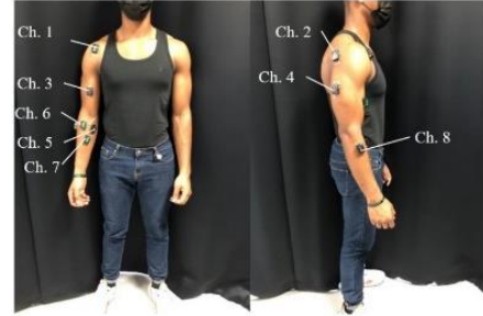
Fig. 5. The EMG placement on a healthy subject.
