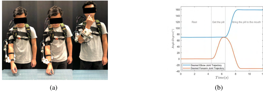
Fig. 8: The ADL task of the experiment: Medication taking. (a) The ADL motion starts with 1) rest, then 2) get the pill, and 3) bring the pill to the mouth. (b) The elbow and forearm trajectory corresponding to the motions.
