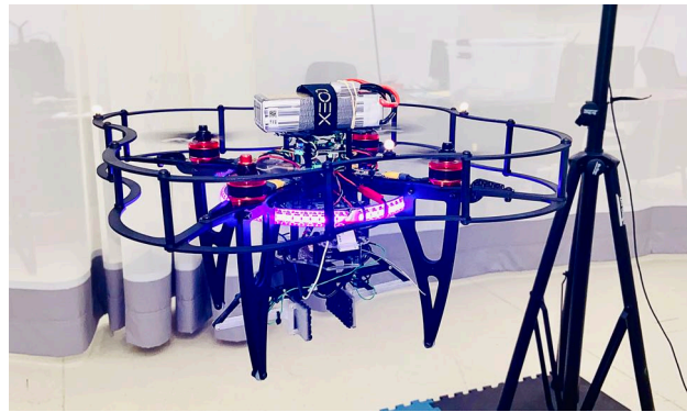
Fig. 1. COEX Clover 4.2 with linkage gripper in flight.
