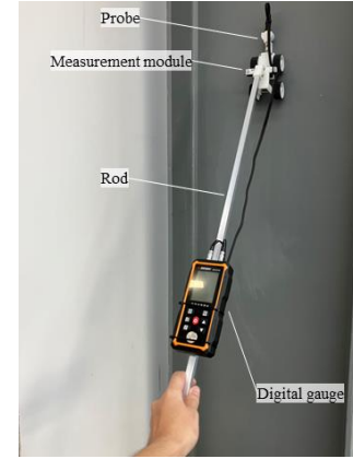
Fig. 8. Measurement module with the rod.
