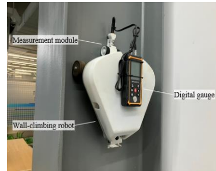
Fig. 11. Robot with the measurement module.
