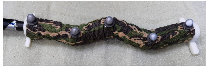
Fig. 1. An overview of the snake robot locomotion experiment. The snake robot is moving on granular terrain. The robot is driven by a single dc motor to generate sidewinding locomotion. The motion data is captured by the motion capture system through five reflective markers on the snake robot.
