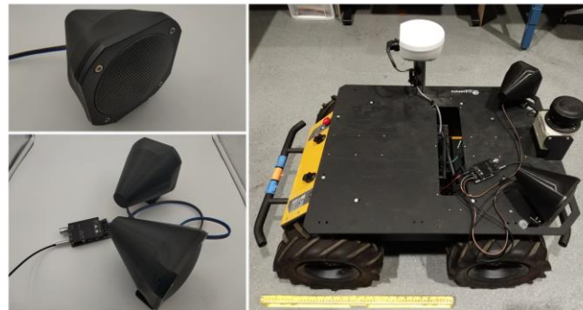
Top Left: a single speaker Bottom Left: the prototype audio system, unmounted Right: the prototype mounted on the Husky robot
