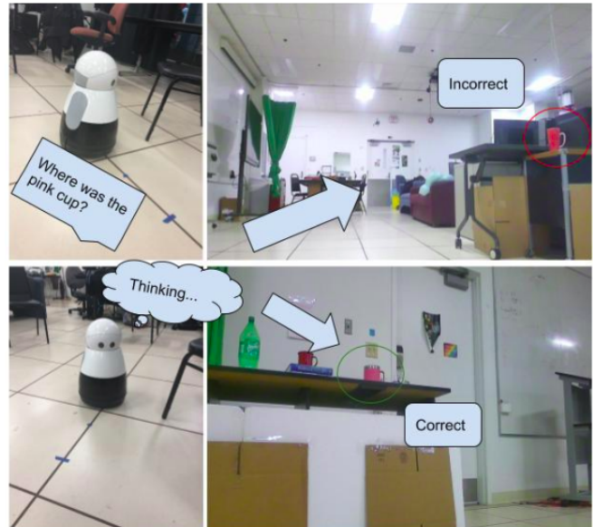
Fig. 1. Our mobile robot deployed with RoboMem monitors the environment for days. When asked about spatial-temporal queries about the objects, it has seen before; it returns a small set of candidate key frames, associated time intervals, and location in the map of the objects seen in the past. The first two candidate images are shown on the right. The top right image is the first ranked candidate image and does not contain our object of interest while the second-ranked image - bottom right correctly contains the object (pink cup)
