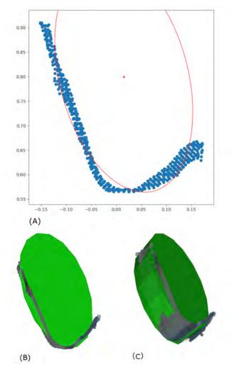
Fig. 3. The elliptical cylinder is generated from a segmented 3D point cloud. For this purpose, the points have extracted that lie in the area where the manipulator is to be applied. (A) These points are projected onto a 2D plane. An ellipse is fitted into this plane. Its ellipse parameters are used to generate an elliptical cylinder, which is used as a model of the human body. In (B), (C) this is fitted into the segmented and cropped point cloud.
