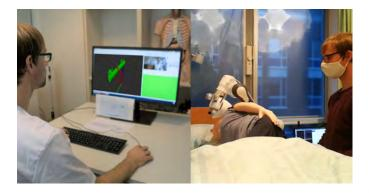
Fig. 2. The system we proposed consists of a remote nurse, who determines the position where the robot is applied to the patient, and an on-site caregiver, who now has both hands free for his work.
