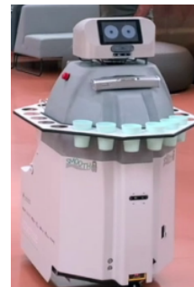
Fig. 1. SMOOTH robot with an add on tray module for serving drinks
