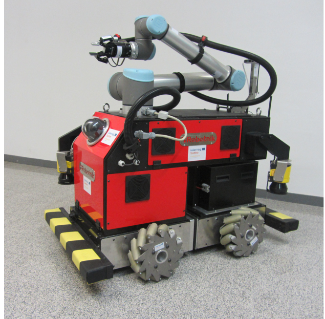
Fig. 1. Prototype of a mobile robotic collaborative manipulator named Campero . This platform is now commercially available as the model RB-EKEN BASE , by Robotnik Automation [10]. A UR10 collaborative arm with an Intel RealSense D435 camera is installed on top of the mobile platform, which also carries two laser scanners Sick S300 and a Axis M5525-E PTZ camera, among other equipment. The setup we envision consists of multiple Campero manipulators with cameras in hand.
