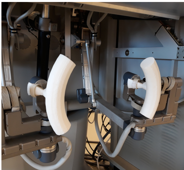
Fig. 3. The da Vinci MTMs with the 3D printed steering wheel segments, push-fitted and fixed by the built-in hook-and-loop fasteners. Using impedance control, the arms are mimicking the behavior of steering wheels, and rotate around a virtual axis.
