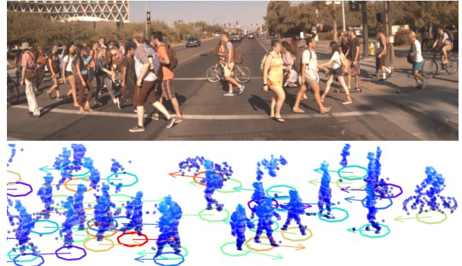
Fig. 1. Association and tracking of pedestrians is challenging in dense, urban environments. We propose a real-time learned association and tracking system with IMM filtering that incorporates LiDAR + camera modalities and show improvements on the task of both association and state estimation.
