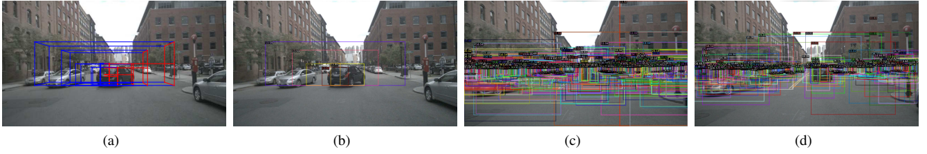
Fig. 3: Radar-based proposals. (a): 3D anchors for one radar detection ( r = 90^\circ ). (b): 2D proposals obtained from 3D anchors. (c): 2D proposals for all radar detections inside the image. (d): Refined radar proposals after applying box regression. Radar-based distances in meters are shown on the bounding boxes.
