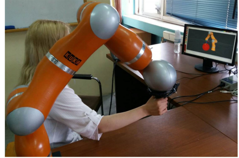
Fig. 3. User manipulates the master KUKA, and the slave KUKA is simulated in the Rviz.
