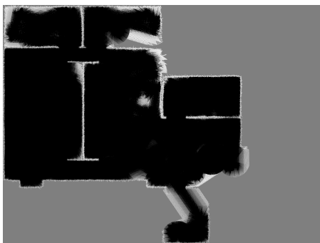
Fig. 13: Map of the autonomy laboratory environment (Figure 4d) generated by robots performing a SLW.
