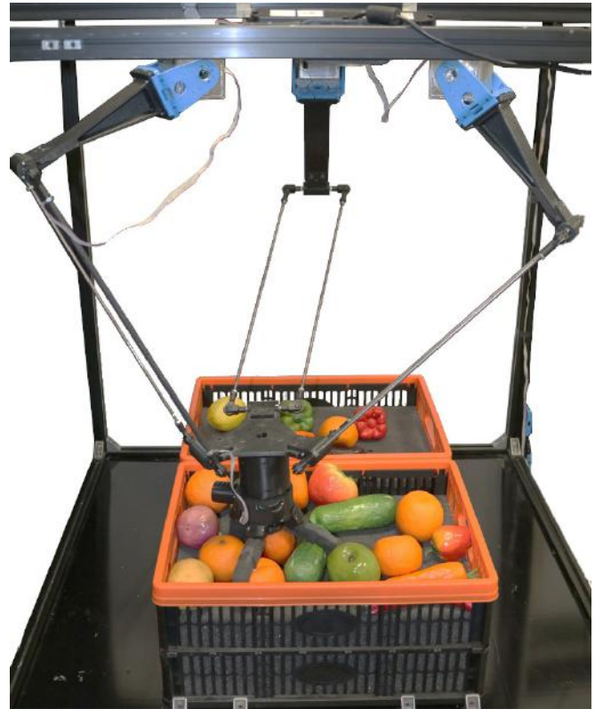
Fig. 1. The SoftHandler: a soft articulated robotic system integrating a parallel delta manipulator, the SoftDelta, and a four fingers gripper, the Pisa/IIT SoftGripper.
