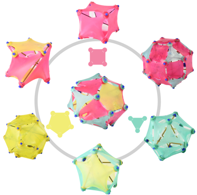
Fig. 1. With square, triangle, and pentagon -shaped membrane actuators as building blocks, we can construct a variety of polyhedra tensegrities. Based on their face arrangement and shapes, tensegrities may be created to more accurately roll on specified paths.
