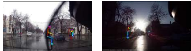
Fig. 8: Examples of OpenPose false alarms, where a windshield wiper and a person on the billboard were mis-identified as pedestrians (top) and tree branches were mis-identified as pedestrians due to dark shadows under glare (bottom).
