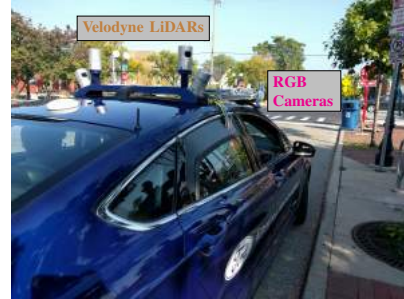
Fig. 2: The PedX data collection system on an autonomous vehicle, parked at an intersection in downtown Ann Arbor, MI, USA.
