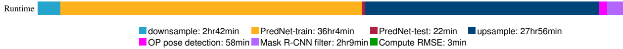
Fig. 5: Computation time analysis for the JAAD dataset experiments, trained and validated on 73,626 frames, tested on 8,280 frames.
