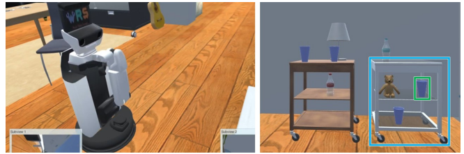
Fig. 2: Left: Typical scene in which the DSR is observing everyday objects. Right: The camera image recorded from the DSR’s position shown in the left-hand panel. The blue and green boxes represent the target (blue glass) and its source (metal wagon). Typical instructions include “Bring me the blue glass next to the teddy bear” and “Bring me the blue glass on the same level as the teddy bear on the metal wagon.”
