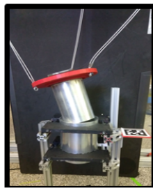
Failed Peg Insertion
