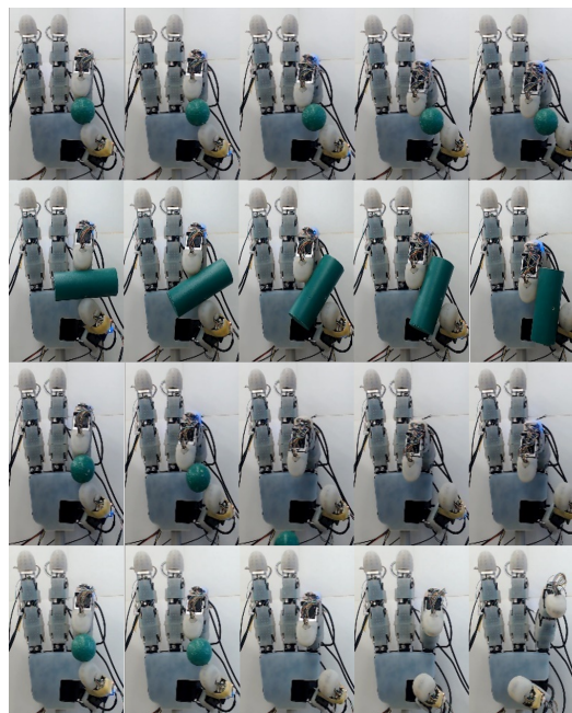
Fig. 6: Top and second rows: For the in-grasp manipulation with architecture I, the object was successfully manipulated. Third row: For the in-grasp manipulation with architecture II, the manipulated object was dropped on the way to the final grasping posture. Bottom row: in-grasp manipulation with architecture IV, the object dropped, and the final posture was wrong. (Grasping postures start from the left side.)
