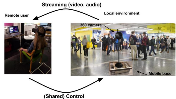
Fig. 1. An illustration of telepresence in which the robot is equipped with a 360 camera and the user with an HMD. The left picture was taken during our user study.
