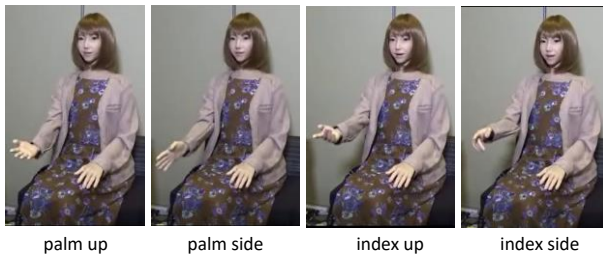
Figure 8. Snapshots of created hand shapes and orientations: palm up, palm to the side, index finger up, and index finger to the side
