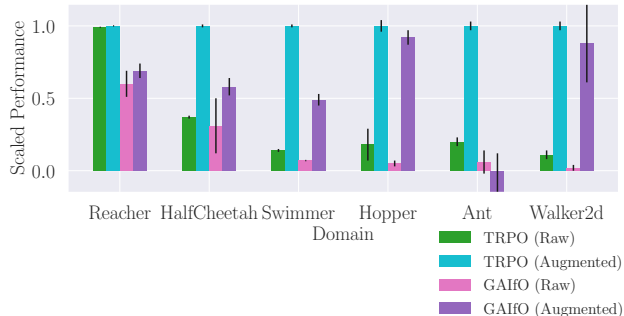
Fig. 2. Quantitative exhibition of the importance of an augmented state space for high performance on six MuJoCo domains for GAIfO and TRPO. Mean and standard deviations are over 100 policy runs. Both methods use a neural network parameterized policy.
