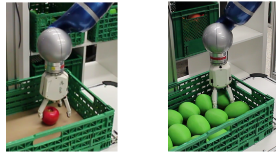
(a) Position Uncertainty (b) Clutter Fig. 14: Use of variable stiffness for grasping (Section IV-B).
