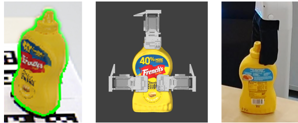
Fig. 6: Refined estimates using RIR (left), retrieved annotated grasps (mid) and successful grasp attempt (right).
