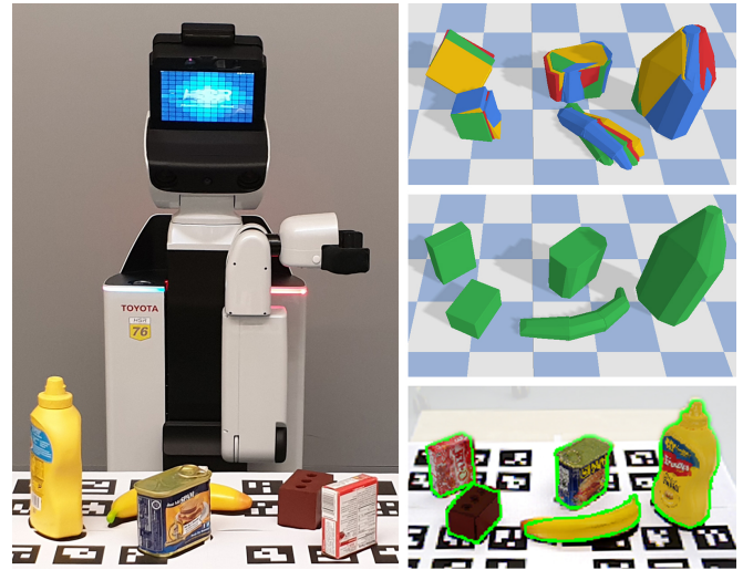
Fig. 1: Grasping YCB-VIDEO objects with a Toyota HSR. Initial pose estimates using [4] in simulation environment (top) are improved using VeREFINE (mid and bottom).
