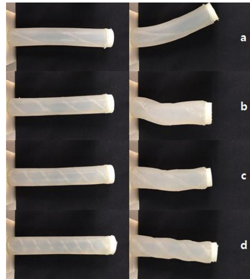
Figure 6. Torsional motion of prototyped soft actuator. (a) Constant pitch ( p = L ) (b) Constant pitch ( p = L/2 ) (c) Constant pitch ( p = L/3 ) (d) Constant pitch ( p = L/4 )
