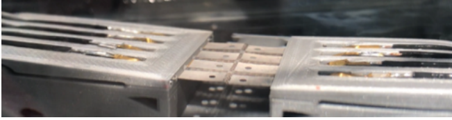
Fig. 7. Assembled open pump design with distributed IPMC actuator coupled to the clamping system.
