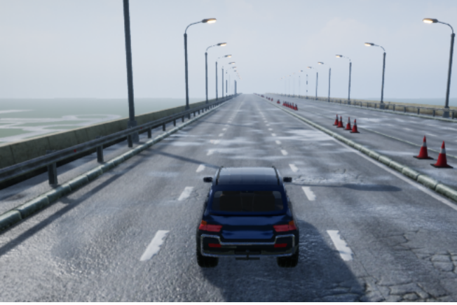
Fig. 3: The simulation with a realistic visual environment for collecting vehicle state variable (lateral position error with respect to the road center).
