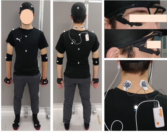
Fig. 3: Motion capture markers (23 in total), Pupil Core eye tracker, and Shimmer3 GSR+ Unit for GSR and PPG.
