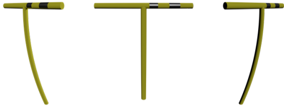
Fig. 2. These objects have the same orientation relative to the rendered fisheye image frame but different translations, resulting in drastically different apparent orientations. Also, objects appear more distorted as they move from the image center.
