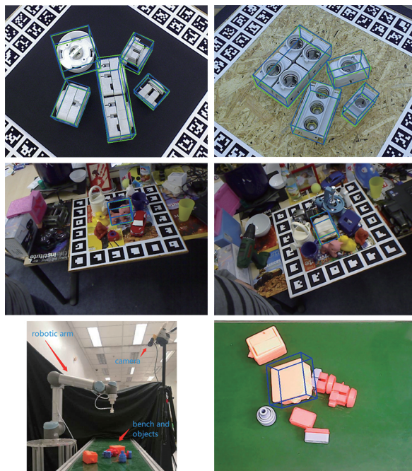
Fig. 4. Visualization of estimated poses of several testing images from T-LESS and LINEMOD (Row 1&2), and a grasping task (Row 3). The grasping setting is shown on the left. The green boxes and blue boxes are ground truth poses and our estimation, respectively. Our network works robustly in these diverse environments.
