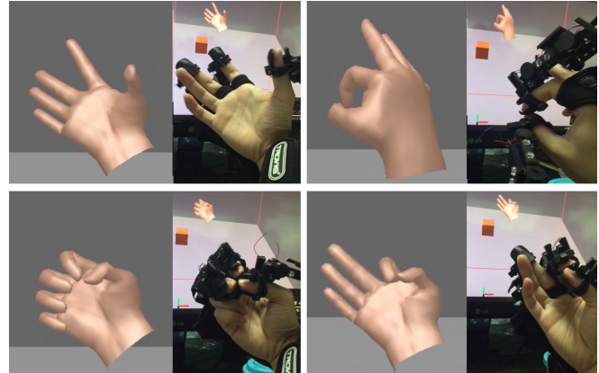
Fig. 1: Hand poses rendered using the fingertip positions from a wearable fingertip tracking device.
